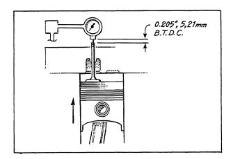
(k) measuring device (Diesel Kiki #57828-3520) in the bolt hole of the injection pump distributor head. (Refer to step c.) Insure that the feeler needle of the measuring device is in contact with the plunger inside of the pump. Zero the measuring device scale.
