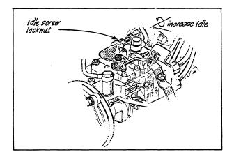
Inspecting and adjusting injection pump timing 3.
