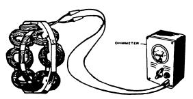
OHMMETER RESISTANCE BETWEEN F1 AND F2 SHOULD BE 12.2 OHMS (± 10%)
