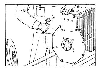
17. Install the flywheel. Install the flywheel onto (a) the rear end of the crankshaft. Install tabwasher (b) the plate (PN 31166) and the flywheel bolts and torque the Bend the tabwasher to bolts. lock the bolts in place.
