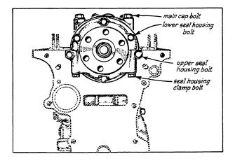
(c) Press the remainder of the seal wick into the groove starting from the center and working outwards.(d) Using a suitable round bar, roll and press the seal into
