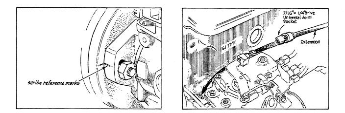
(d) Mount the injection pump on the gear case, then tighten the pump drive gear attaching nuts.
