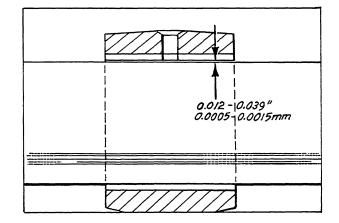
Small end bushing replacement 4. (a) Using a press, press out the bushing. (b) Align the oil passages of the connecting rod and the small end bushing; press in the bushing to the connecting rod bore. After a small end bushing (C) has been replaced, ream the bushing bore to obtain the specified clearance between the the small end bushing and
