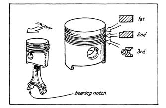
(c) Install the piston rings to ring grooves on the piston with the inscription mark on ring upward.
