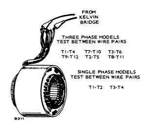
FIGURE 18. TESTING STATOR WINDINGS
