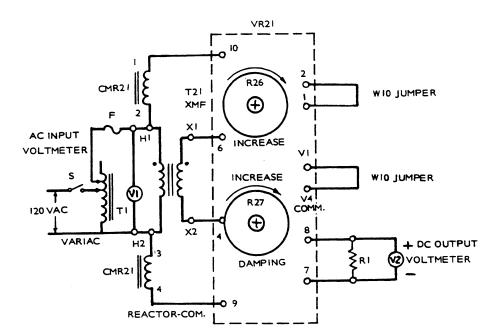
FIGURE 7. VOLTAGE REGULATOR CHECKOUT TEST EQUIPMENT CONNECTIONS
