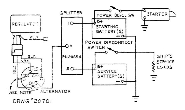
NOTE: On Alternators which have an isolation diode between their output and regulator terminals, such as the Motorola units used with most WESTERBEKE engines, the regulator wire should be removed from the REG terminal and reconnected to the OUTPUT terminal as shown. The diode in the splitter will provide an equivalent voltage drop.
