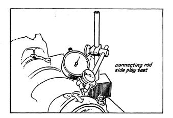
5. Inspecting connecting rod side play Check the connecting rod side play with the dial gauge and, if it exceeds the limit, replace the connecting rod and crankshaft.
