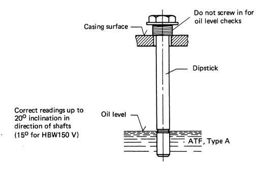
To check the oil level, just insert the dipstick; DO NOT SCREW IN. Retighten the hex screw with the dipstick after the oil level check. Do not omit the o-ring seal.
