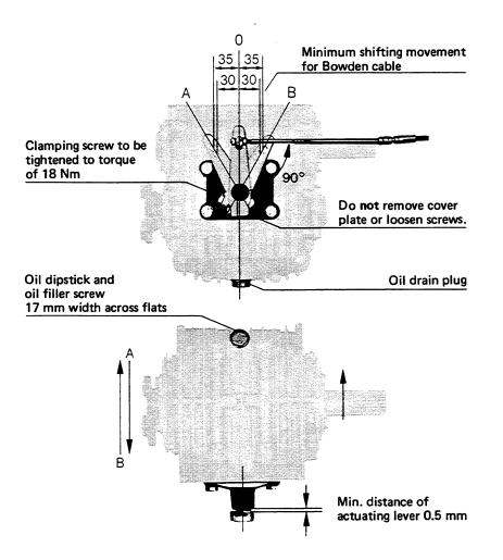
The position of the cover plate underneath the actuating lever is factory-adjusted to ensure equal lever travel from neutral position to A and B. Therefore, do not loosen the capscrews mounting this assembly.
