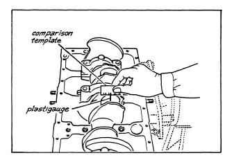
Connecting rod cap Tightening torque: 7.8-8.0 m-kg (56-58 ft-lb)
