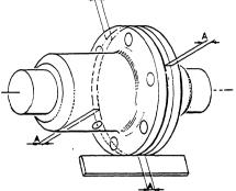
90° between each position. This test will also check whether the propeller half coupling is in exact alignment on its shaft. Then, keeping the propeller coupling in one position, the alignment should be checked rotating the engine half coupling to full position each 90° from the next one.
