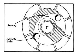
(e) With the use of extractor #49 SE01 157 apply sufficient pressure to loosen the pump from the keyed gear. The loose hold down nuts will prevent the pump from falling from the engine.
