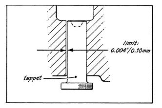
2. Inspecting clearance between tappet and tappet bore Check the clearance between the tappet and tappet bore and, if the clearance is greater than the limit, replace the tappet or cylinder block.
