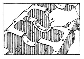
(d) Fit the thrustwasher to the main bearing cap so that the oil grooves on thrustwasher face to crankshaft side. Then install the main bearing cap to the cylinder block with arrow mark of the main bearing cap facing the crankshaft pulley side.
