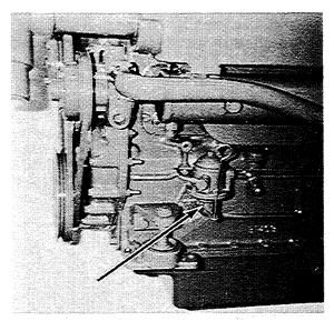
Typical Mechanical Fuel Lift Pump
