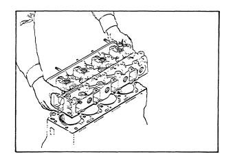
(c) Remove the push rods. Label each rod as to which valve it belongs.
