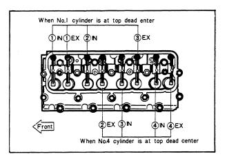
AFTER THE ENGINE HAS BEEN REASSEMBLED, WARM UP THE ENGINE AND READJUST THE VALVE CLEARANCES.
