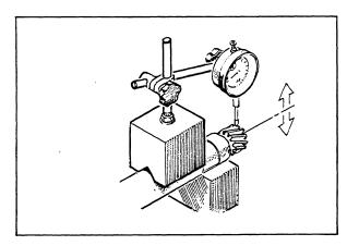
Clearance between pump body and shaft Measure the above clearance with a dial gauge and magnet base.
