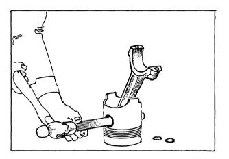
Note: If the piston pin is tightly fitted, heat the piston head with the aid of a hot plate or similar device.
