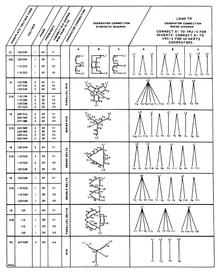
FIGURE 6. GENERATOR WIRING AND RECONNECTION DIAGRAMS
