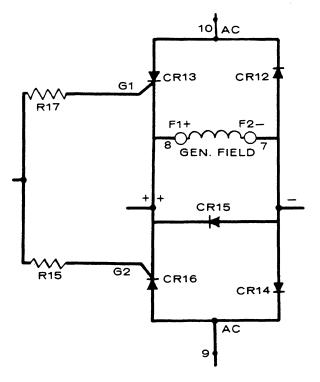
FIGURE 10. SILICON CONTROLLED RECTIFIER BRIDGE
