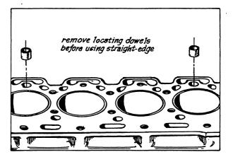
Distortion inspection Check the gasket face distortion of the cylinder block and if it exceeds the limit, repair or replace it.
