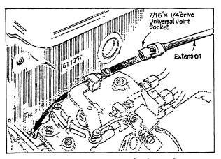
(c) Remove the nut (4) and lockwasher (5) from the injection pump shaft.
