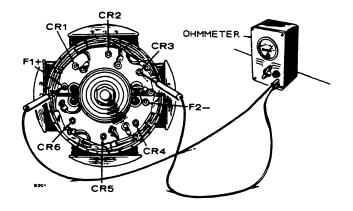
FIGURE 9. TESTING ROTATING RECTIFIERS
