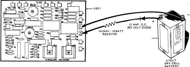
FIGURE 8. FLASHING THE FIELD
