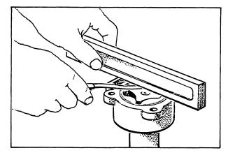
Free length of plunger spring Check the relief valve for worn plunger and fatigued spring.
