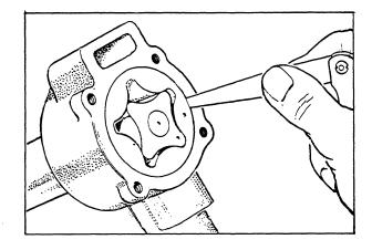
4. Clearance between outer rotor and pump body Check the clearance between the outer rotor and pump body with a feeler gauge. If the clearance exceeds the limit, replace the rotor or pump body.
