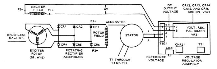
FIGURE 22. GENERATOR-REGULATOR ELECTRICAL SCHEMATIC
